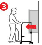
(3) Adjust the support so that the oven is resting on the beam and not the cabinet. Use the AllDolly to pull oven 3/4 of the way out (about 16")
