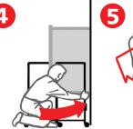
(4) Swing/rotate one leg along side the oven and slide short beam up until it supports the oven. Repeat with the other side.
